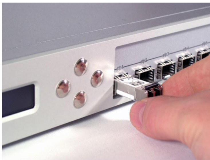
Figure 2.2. Installing a 1000 Base LX/SX Module
