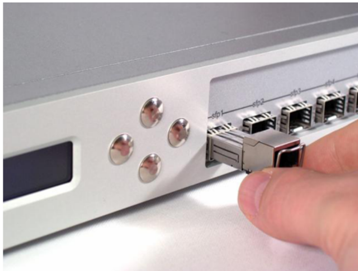
Figure 2.4. Installing a 1000 Base TX Module
