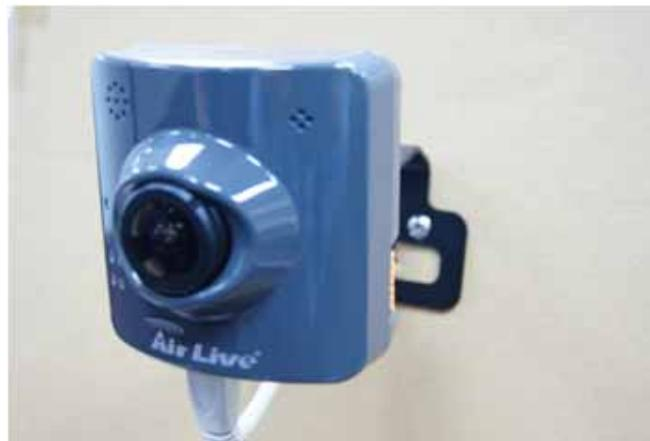
4. You can adjust the silver screw to fix the angle of camera.
