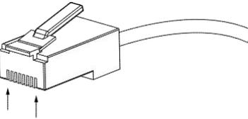
Figure 3-3 RJ-45 connector of the console port
