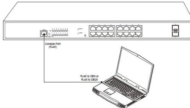
Figure 3-4 Connecting the console port of S2518PB and computer
