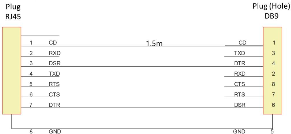
Figure 3-5 Cable connection at the console port
