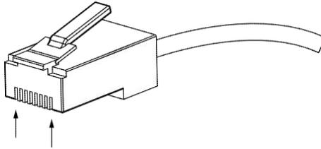
Figure 3-7 RJ-45 connector of the console port
