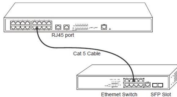
Figure 3-8 Connecting 10/100/1000Base-T ports and other Ethernet terminal
