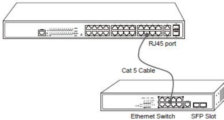
Figure 3-8 Connecting the 10/100 Base-TX port and other Ethernet terminals
