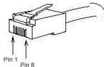
Figure 3-6 RJ-45 connector of the console port
