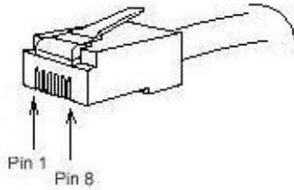
Figure 3-3 RJ-45 connector of the console port
