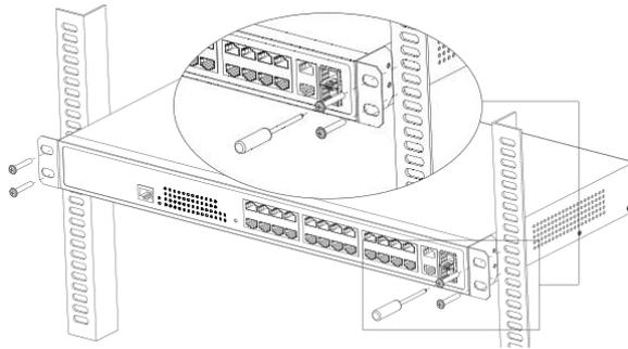
Figure 3-2 Installing the switch on the cabinet
