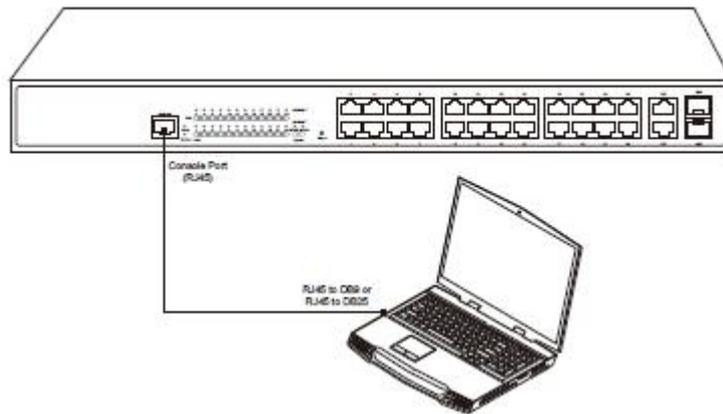
Figure 3-4 Connecting the Console port and the PC of the S2226PB switch
