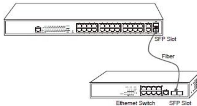
Figure 3-6 Gigabit optical ports and other switches
