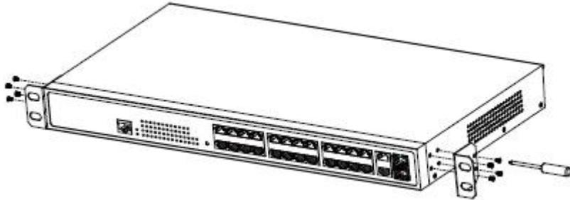
Figure 3-1 Fixing the machine box of the switch
