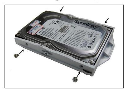
b. If you are using 2.5" hard disks, align the hard disk with the 4 smaller holes on the hard disk tray, and secure the hard disk from the bottom with the screws (for securing 2.5" hard drives) provided.
