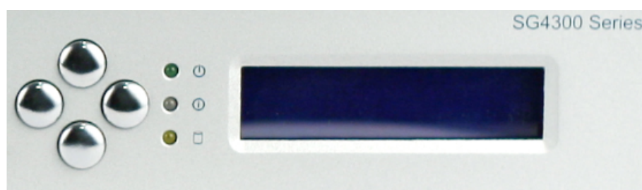
Figure 1.3. The SG4300 Series Keypad and Display
