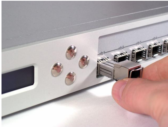
Figure 2.4. Installing a 1000 Base TX Module
