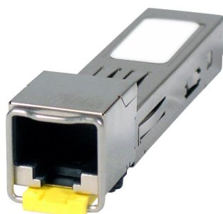
Figure 2.3. A typical 1000 Base TX module
