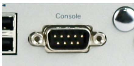
Figure 2.5. The SG4300 Series RS-232 Console Port
