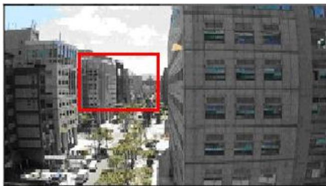
Users can configure up to 10 sets of Motion Detection Windows in each set of Motion Detection Setting. Click on the <add> button under the Live Video Pane to add a Motion Detection Window. To cancel a Motion Detection Window, move the mouse cursor to the selected Window, and click on the <delete> button.
