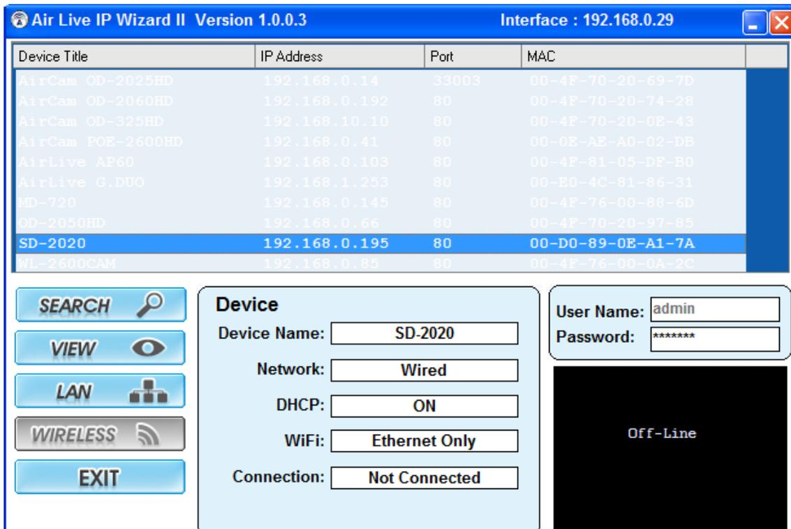
5. If the Camera's IP address is in the same IP segment as your LAN, select the founded IP Camera and double click on the item. Then, the default browser will show up and connect to the IP camera's Web automatically.
