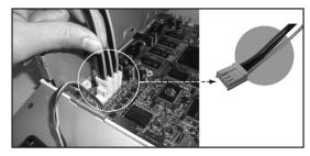
6 Connect the 4 SATA cables. The longest one should be connected to the HDD 1 connecter.
