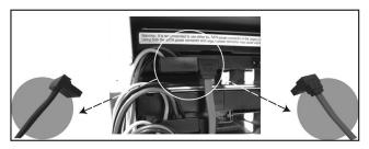
10 Use the cable ties to arrange the hard disk power cables and SATA cables.
