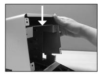
Fix the cable lock to its hole on the back cover. Make sure on the inner side of the back cover, the cable lock is hooked.
