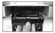
8 Fix the hard disks with the 5mm screws provided. Use 2 screws on each side of the hard disk.
