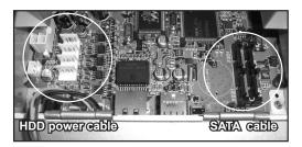
5 Connect the 4 hard disk power cables.
