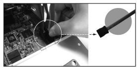
Place the hard disks into the hard disk tray with connectors faced outside. The top hard disk is HDD 1, and then HDD 2, HDD 3, and HDD 4.
