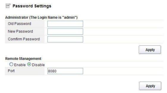
You could choose to enable or disable Web Server Access on WAN. If you enable this function, you can manage the router remotely.
