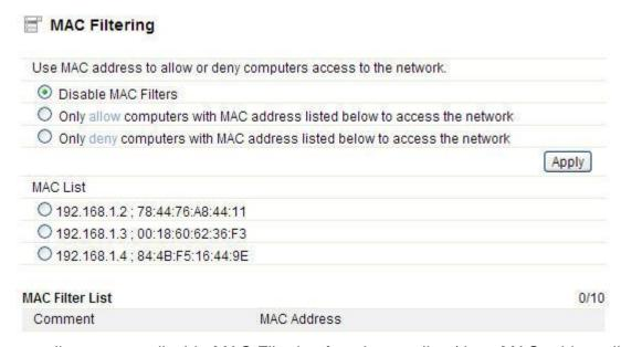
This router allows you to disable MAC Filtering function or allow/deny MAC address listed.
