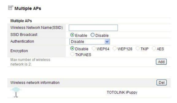
Wireless Network Name (SSID): define one more SSID for your WLAN.
