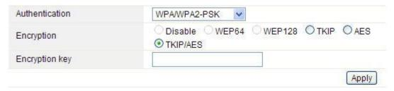
**Note:** Since WEP has been proved vulnerable, you may consider using WPA2 for the most secure connection. You should select the appropriate security mechanism according to your needs. No matter which security suite you select, they all will enhance the over-the-air data protection and/or privacy on your wireless network.
