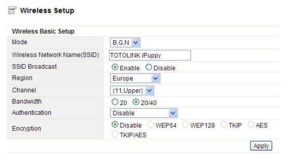
**Mode:** This option allows you to choose the radio standard for operation of your Router. 802.11b and 802.11g are old 2.4GHz mode, while 802.11n is the latest standard based on faster Orthogonal Frequency Division Multiplexing (OFDM) modulation. Here, by default, the B, G, N Mode is selected, this mode offers better compatibility.
