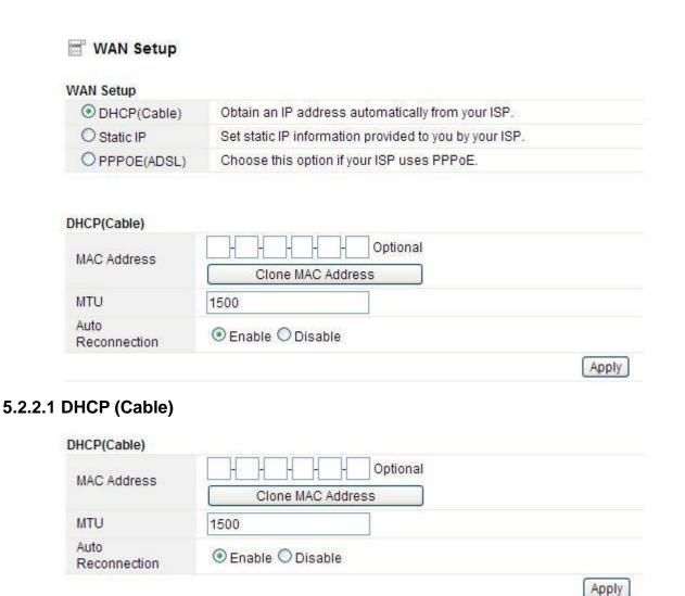
**MTU:** It means Max Transmit Unit for packet. When using slow links, large packets can cause some delays thereby increasing lag and latency. The default value is 1500.
