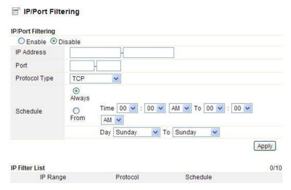
You can select to enable or disable IP/Port Filtering function. By default, it is disabled.
