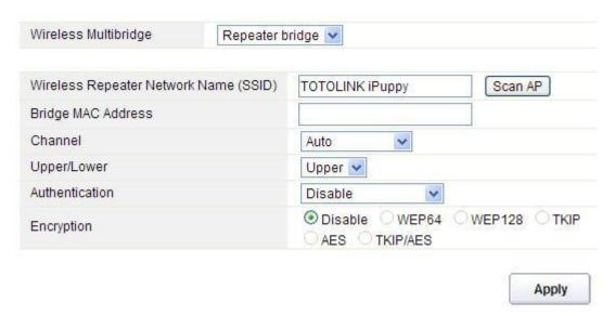
Wireless Repeater Network Name (SSID): choose the SSID you want to implement the repeater function.
