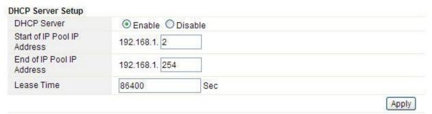
**Start of IP Pool IP Address:** displays the start IP Address of the range that will be assigned to each computer connected with the router.
