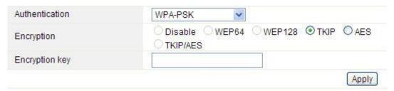
**WPA2:** it means Wi-Fi Protected Access 2, it is the current most secure method of wireless security and required for 802.11n performance. This mode allows you to choose **TKIP+AES** Algorithm. If you choose Enterprise related modes, you are required to enter **RADIUS Server.**
