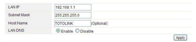
**IP Address:** This is the IP addresses to be represented by the LAN (including WLAN) interface that is connected to the internal network. This IP will be used for the routing of the internal network (it will be the Gateway IP for all the devices connected on the internal network).
