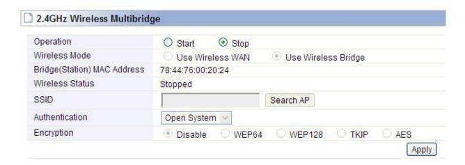
Wireless Bridge: In this mode, the router is used as an AP to get other router's signal.
