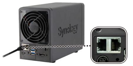
2 Connect the AC adapter to the power port of the DiskStation. Connect one end of the AC power cord to the AC power adapter, and the other to the power outlet.
