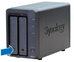
2 Pull the hard drive tray handle in the direction as indicated below to remove the hard drive tray.
