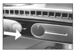
2. Pull the clip in the direction as indicated below to remove the hard disk tray.
