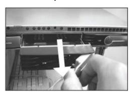
3. Attach the prepared SATA hard disk to the hard disk tray and use 4 screws to fix the hard disk. Refer to the picture below for the screw position
