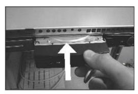
5. Push the clip to fix the hard disk tray.
