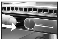
Pull the clip in the direction as indicated below to remove the hard disk tray.
