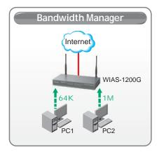
The gateway also supports bandwidth management function. So you can control the **speed** of the user's account. The Firewall management allows you to define different service type. For example, administrator can define the firewall so only web and email service is possible. Administrator can also restrict users by using MAC access control for up to 40 entries.
