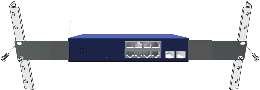
Figure 14: Installing the Switch in a Rack
