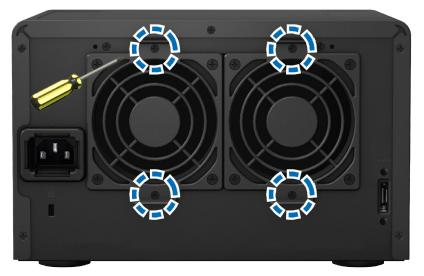
4 Remove the malfunctioning fans by disconnecting the fan cable from the connectors.
