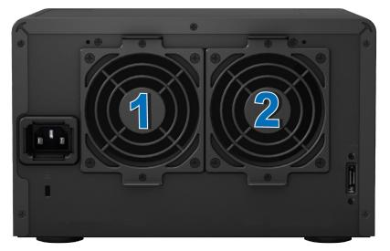
3 Remove the screws that secure the fan panels and pull the panels from the expansion unit.
