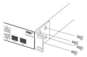
Figure 3-2 Attaching the Brackets
