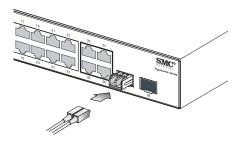
Figure 4-3 Making Fiber Port Connections
