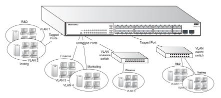
Figure 2-5 Making VLAN Connections
