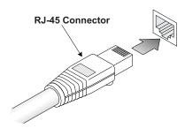
Figure 3-1 RJ-45 Connections
