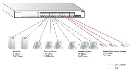
Figure 2-2 Collapsed Backbone
