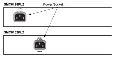
Figure 1-4 Power Supply Socket
