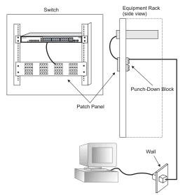
Figure 4-2 Network Wiring Connections
