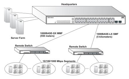
Figure 2-4 Remote Connection with Fiber Cable
