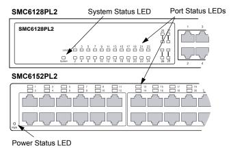
Figure 1-3 Port and System Status LEDs
