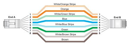
Figure B-2 Straight-through Wiring
