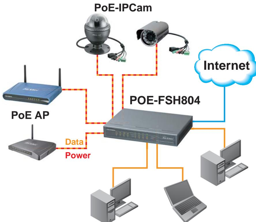
\* Priority: Priority of port 1 is higher than port 2 (port 1 > port 2 > port 3 > port 4). For example, Port 1, 2 and 4 are using 15.4w (maximum power per port is 15.4W), the system power is 46.2w in total (PoE max LED is red ). If there is an additional PD connected to Port 3 with 10W then the system will stop supplying power to Port 4 for protecting the system, this means Port 1, 2 will use 15.4w, and Port3 will use 10w, and system will not supply power to Port 4.
