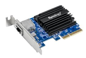
Equipped with an RJ-45 connector and supports IEEE 802.3an/bz (10GBASE-T/NBASE-T) and 802.3x, E10G18-T1 helps you smoothly migrate to a 10GbE networking environment with your existing infrastructure. Supporting backward compatibility and auto-negotiation between 10Gbps, 5Gbps, 2.5Gbps, 1Gbps and 100Mbps data rate, E10G18-T1 is an economic solution to overcome the data transmission bottleneck for small businesses and home users.
