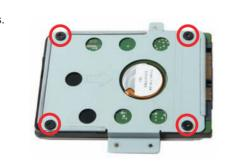
2. As shown, install the HDD & bracket in the chassis and push it towards the direction as indicated by the red arrow to connect the HDD connector.
