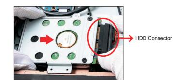
3. Tighten the HDD & bracket with three screws.
