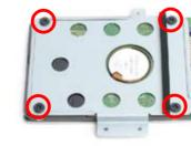
2. As shown, install the HDD & bracket in the chassis and push it towards the direction as indicated by the red arrow to connect the HDD connector.
