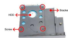
4. As shown, install the ODD/HDD & bracket in the chassis and push it towards the direction as indicated by the red arrow to connect the
