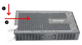
5. Turn your XPC upside down and tighten the ODD/HDD & bracket
