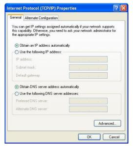
Click "OK", InRouter will allocate an IP address: 192.168.2.x, and a gateway: 192.168.2.1(the default address of IR6x5).
