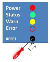
2) When you see ERROR LED turns on (about 10 seconds after power on), release the RESET button:
