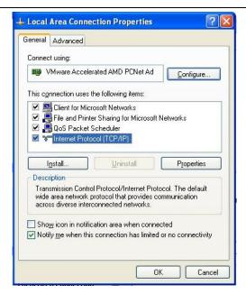
Choose "Internet Protocol (TCP/IP)", click "properties" button, ensure your PC can obtain IP and DNS address automatically. (Or you can set your PC in the subnet: 192.168.2.0/24, for example, set IP: 192.168.2.10, Net Mask: 255.255.255.0, Default Gateway: 192.168.2.1)
