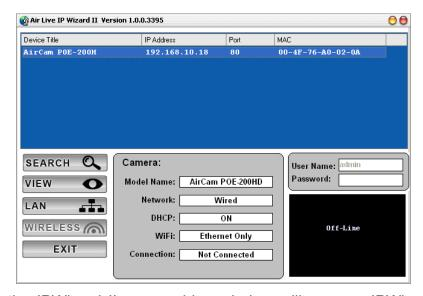
When launch the IPWizard II, a searching window will pop up. IPWizard II is starting to search Network Cameras on the LAN. The existed devices will be listed as below.
