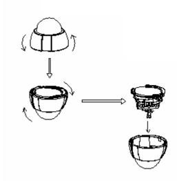
4. For lens adjustment, move the camera body (some model types limits the PCB board to 180° rotational adjustment) and set the focus by turning the lens to the left or right direction. When the camera focus adjustment has been completed, rotate the dome housing clockwise to secure it to the mounting base
