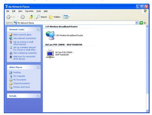
Click the targeted **Device.** Then Internet Explorer will connect to this Network Camera automatically.
