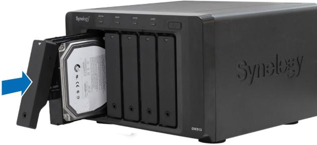
**Important:** Make sure the tray is pushed in all the way. Otherwise, the hard disk might not be able to function properly.
