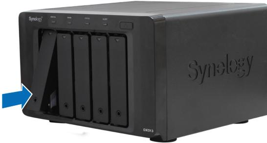
3 Pull the handle to remove the hard drive tray from DX513.
