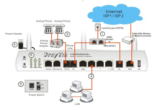
**Caution**: Each of the Phone ports can be connected to an analog phone only. Do not connect the phone ports to the telephone wall jack. Such connection might damage your router.
