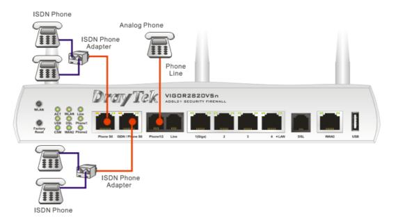
Yet, if the user configures ISDN / Phone S0 as TE Mode in **VoIP>> Phone Settings**, the **green** LED will light on to indicate **ISDN-TE** is selected. Then, the port is specified for ISDN line only. Refer to the following figure for reference.
