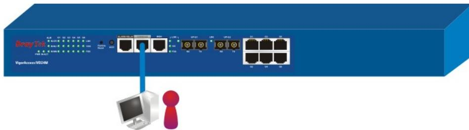
*Figure 2-3. Master console port connection*
