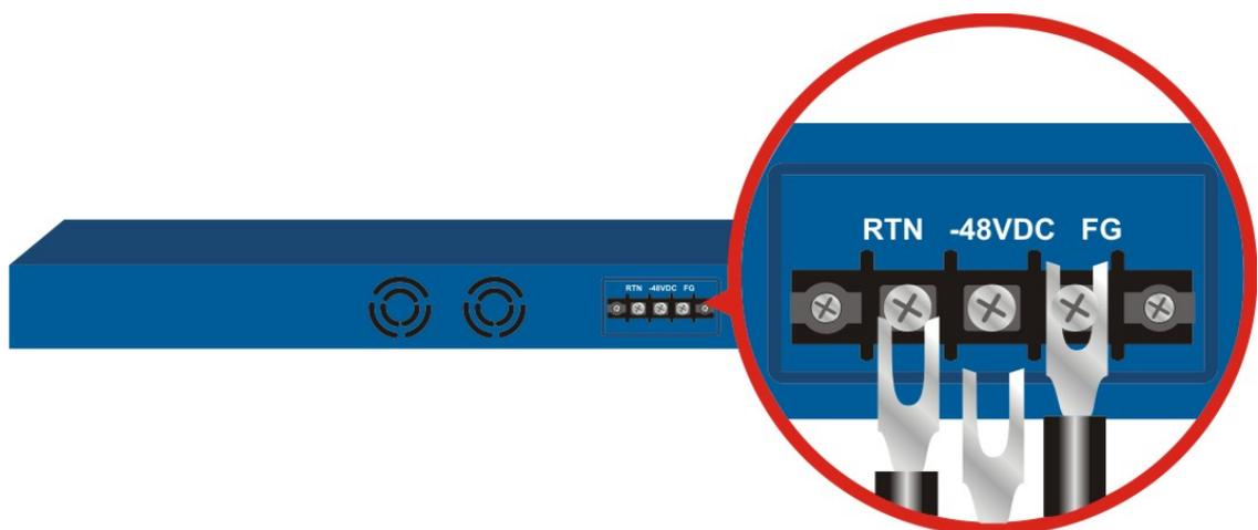
Figure 1-9. Rear panel and DC power input
