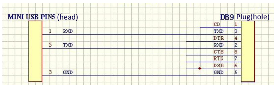
Figure3-4 Cable connection at the console port
