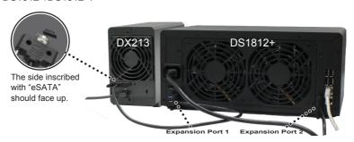
After the connection is complete, DX213 will be turned on or off automatically when the connected DiskStation powers on or off.  $\frac{1}{2} \left( \frac{1}{2} \right) = \frac{1}{2} \left( \frac{1}{2} \right) \left( \frac{1}$
