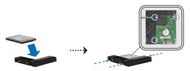
b Slide the 2.5" Disk Holder into the hard drive bay, and push it all the way until the hard disk is connected to the SATA connector. Secure the Disk Holder with the provided screws.
