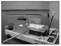
Place the other hard disk in the HDD bay. This disk will be disk No.2 (disk#2).
