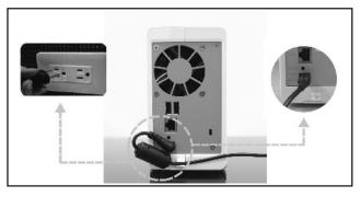
2 Use the LAN cable to connect the server to your switch/router/hub.
