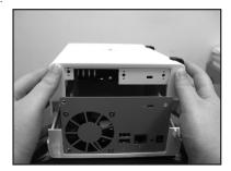
Place the hard disk connected with the shorter HDD Data Cable in the HDD bay. It will be disk No.1 (disk#1).
