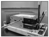
Connect the HDD Data Cables and HDD Power Cables to the motherboard correctly according to the disk number.
