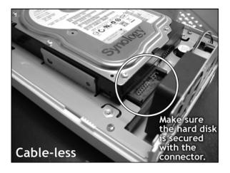
6. Fix the hard disk with the 4 HDD screws provided.
