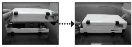
9. Fix the case with the 2 case screws provided.
