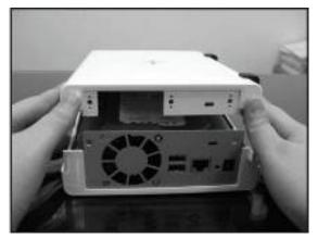
5. Place the hard disk inside the HDD bay.
