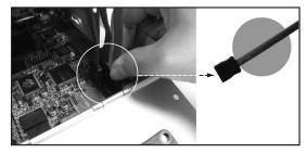
Place the hard disks into the hard disk tray with connectors faced outside. The top hard disk is HDD 1, and then HDD 2, HDD 3, and HDD 4.
