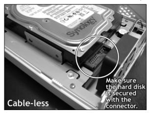
5. Fix the hard disk with the 4 HDD screws provided.
