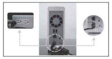
2. Use the LAN cable to connect the server to your switch/router/hub.
