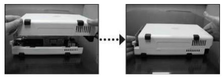
7. Fix the case with the 2 case screws provided.
