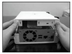
4. Place the hard disk inside the HDD bay.
