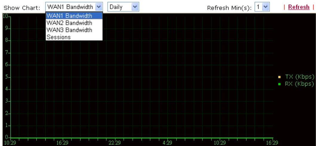
The horizontal axis represents time. Yet the vertical axis has different meanings. For WAN1/WAN2/WAN3 Bandwidth chart, the numbers displayed on vertical axis represent the numbers of the transmitted and received packets in the past.
