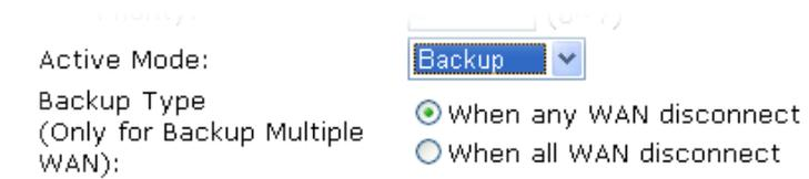
A screenshot of the configuration interface showing 'Active Mode' set to 'Backup' and 'Backup Type' set to 'When any WAN disconnect'.
