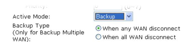
A screenshot of the Backup WAN configuration interface. It shows a 'Priority' field with a value of 0 and '(0~7)' next to it. Below that is the 'Active Mode' dropdown menu, which is set to 'Backup'. Underneath is the 'Backup Type (Only for Backup Multiple WAN):' section with two radio button options: 'When any WAN disconnect' (which is selected) and 'When all WAN disconnect'.
