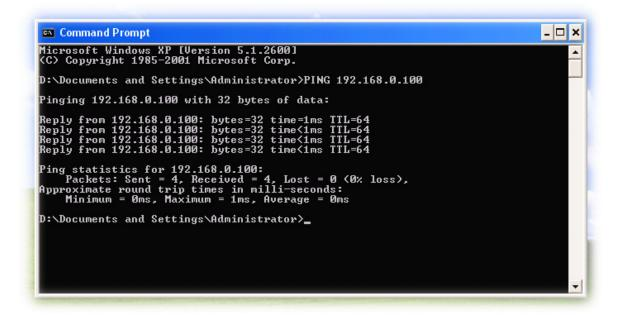
If you want to detect any other devices conflicts with the IP address of Network Camera, also can utilize the PING command but you must disconnect the Network Camera from the network first.
