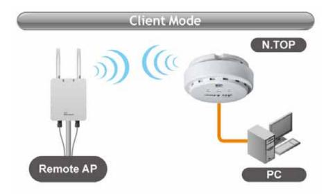
In Client Ad Hoc mode, N.TOP can connect to other wireless adapters without access point. Users can attach a computer or a router to the LAN port of N.TOP to get network access.
